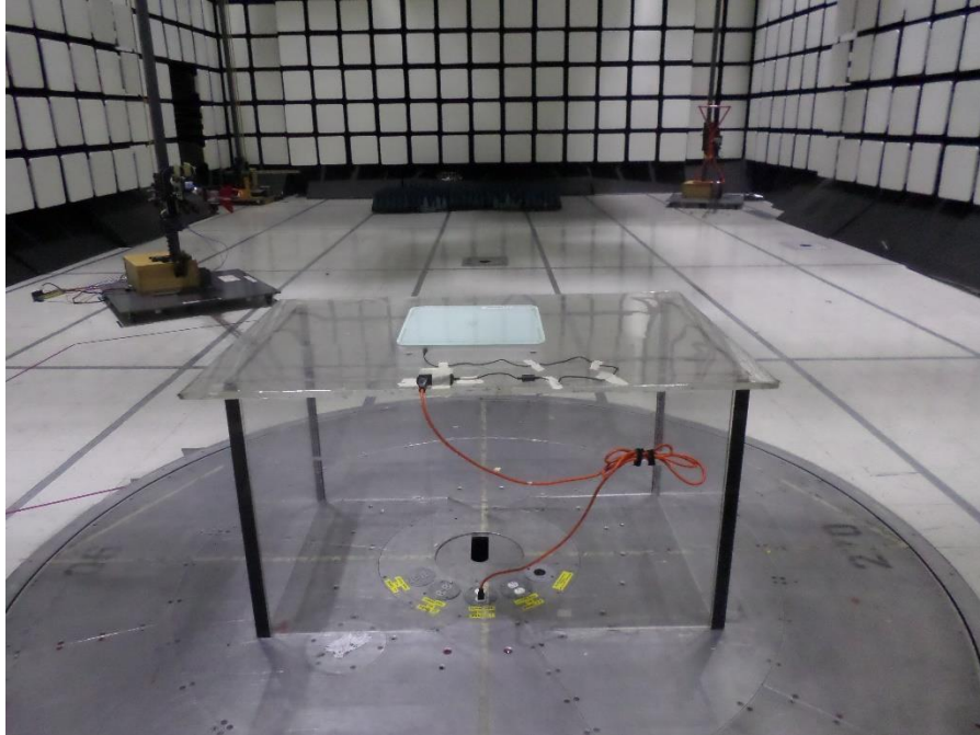
Figure 6: Radiated Emissions - 30-1000 MHz- Setup Rear View
