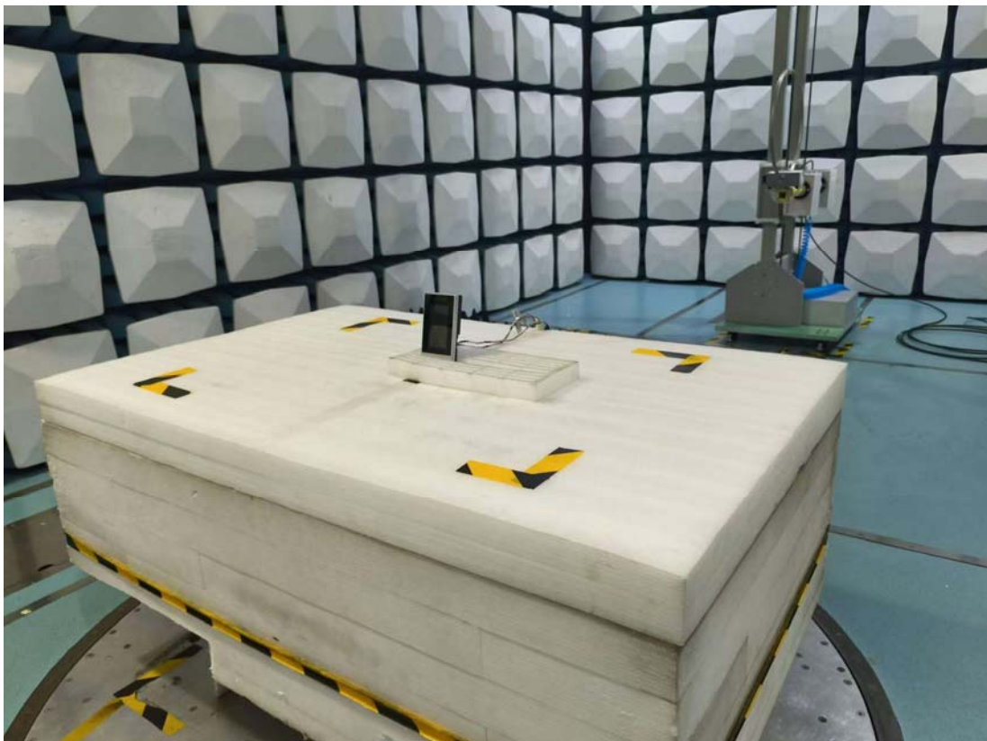
Radiated Emission 9k-30MHz Perpendicular View
