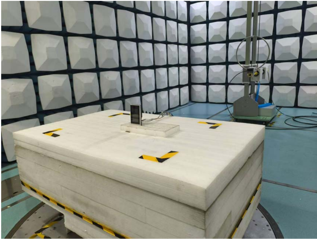
Radiated Emission 9k-30MHz Perpendicular View
