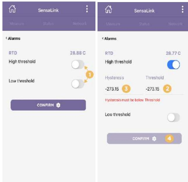
High alarm is enabled when value reaches the high threshold within the increase phase and is disabled when it reaches high threshold hysteresis within the decline phase.
