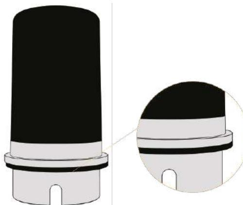
6. Fully tighten the nut ring
