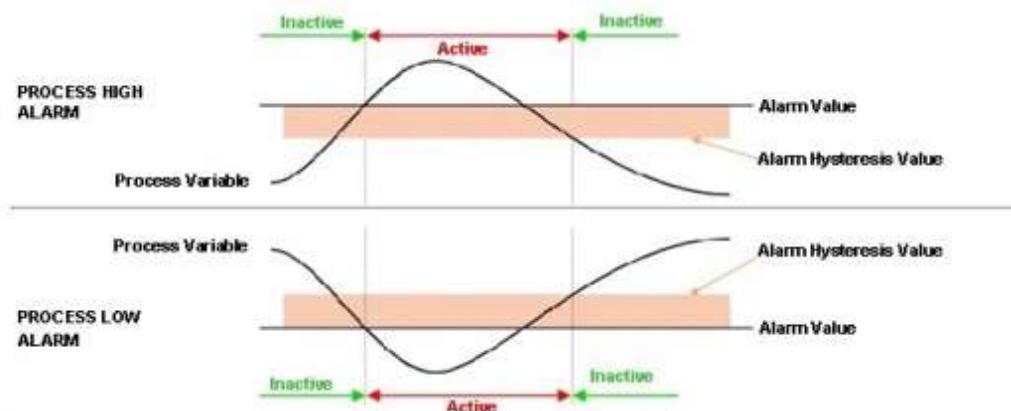
High alarm is enabled when value reaches the high threshold within the increase phase and disabled when it reaches high threshold hysteresis within the decline phase.
