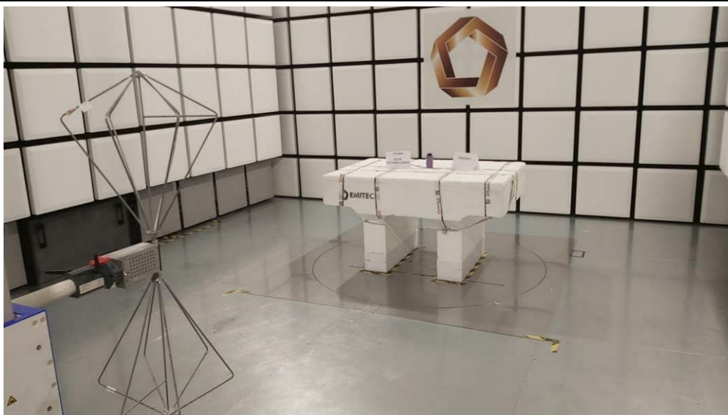
TEST SETUP PHOTO(S) – RADIATED EMISSION LIMITS – 30 MHz TO 200 MHz
