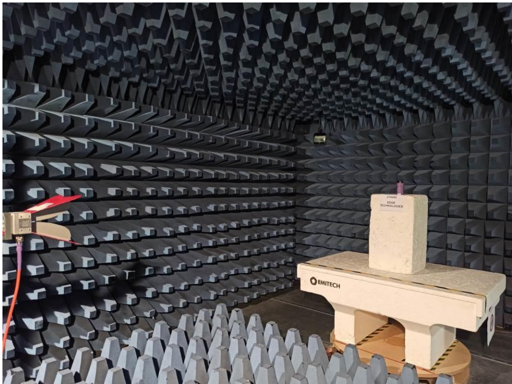
TEST SETUP PHOTO(S) – RADIATED EMISSION LIMITS – 1 GHz TO 10 GHz
