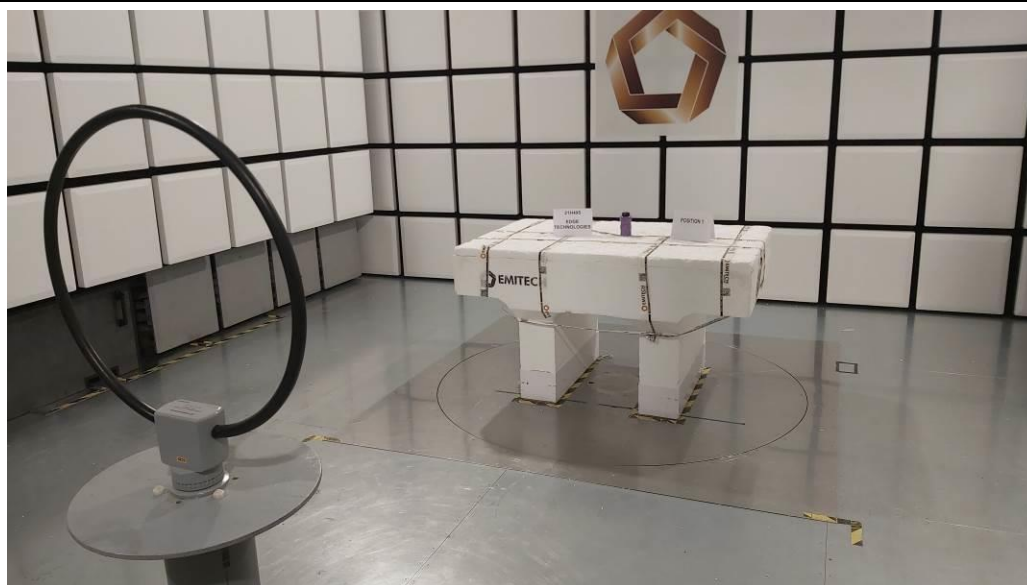
TEST SETUP PHOTO(S) – RADIATED EMISSION LIMITS – 9 KHZ TO 30 MHZ
