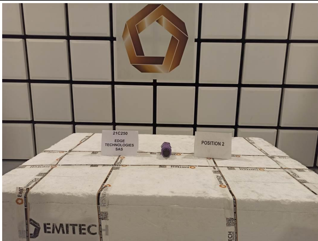
TEST SETUP PHOTO(S) – RADIATED EMISSION LIMITS – POSITION 2
