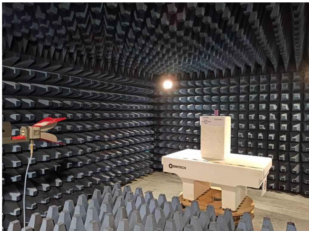
TEST SETUP PHOTO(S) - EQUIVALENT ISOTROPIC RADIATED POWER
