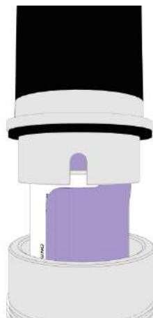
4. Insert the battery inside the electronic cartridge
