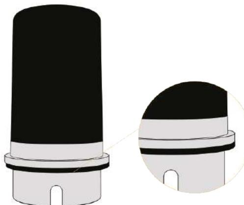
6. Fully tighten the nut ring
