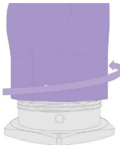
3. Remove the antenna cap carefully without dropping the electronic cartridge.
