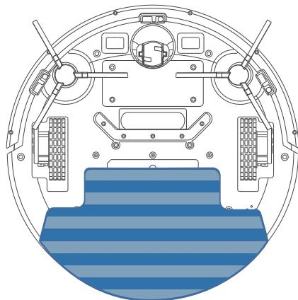
\*The water tank has no function of closing water seepage, and it will start to seep after water injection. Please remove the water tank before charging.
