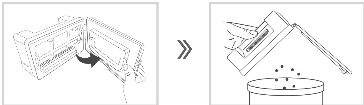
Remove the filter elements. HEPA can be washed with water, and you can tap it to remove dust before washing.
