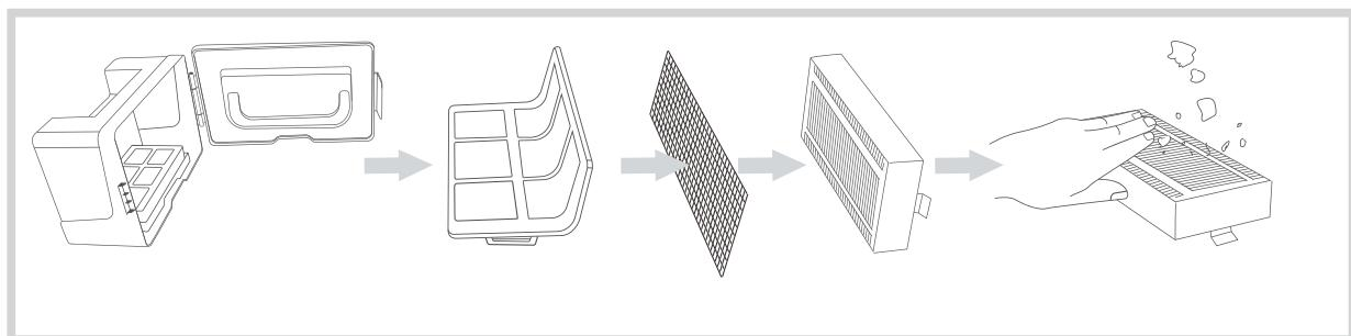
Wash the dust collector and the first filter element, dry the dust collector and filter elements, and keep them dry to ensure their service life
