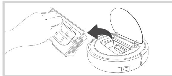
Open the dust collector lock and pour the dust and garbage.
