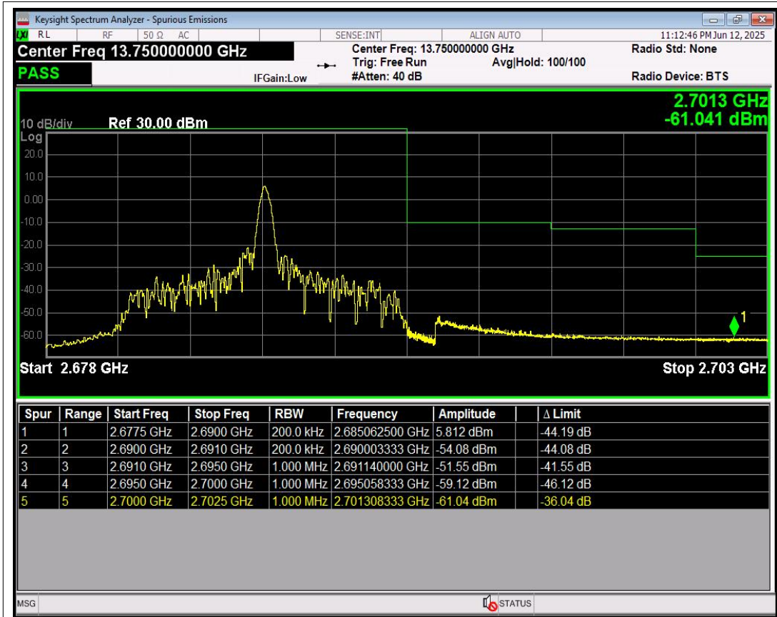
Band41 16QAM BW=10MHz Channel=41540 RB Size=1 Position=#Mid
