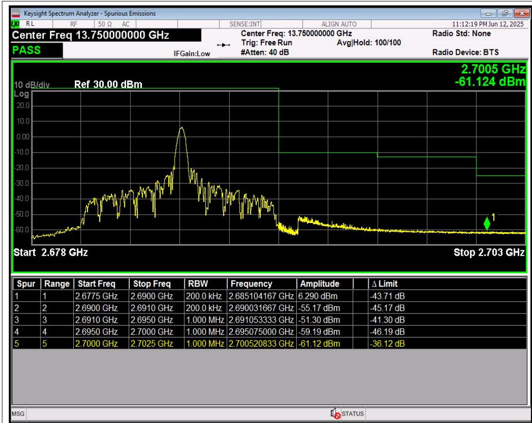
Band41 QPSK BW=10MHz Channel=41540 RB Size=1 Position=#Mid
