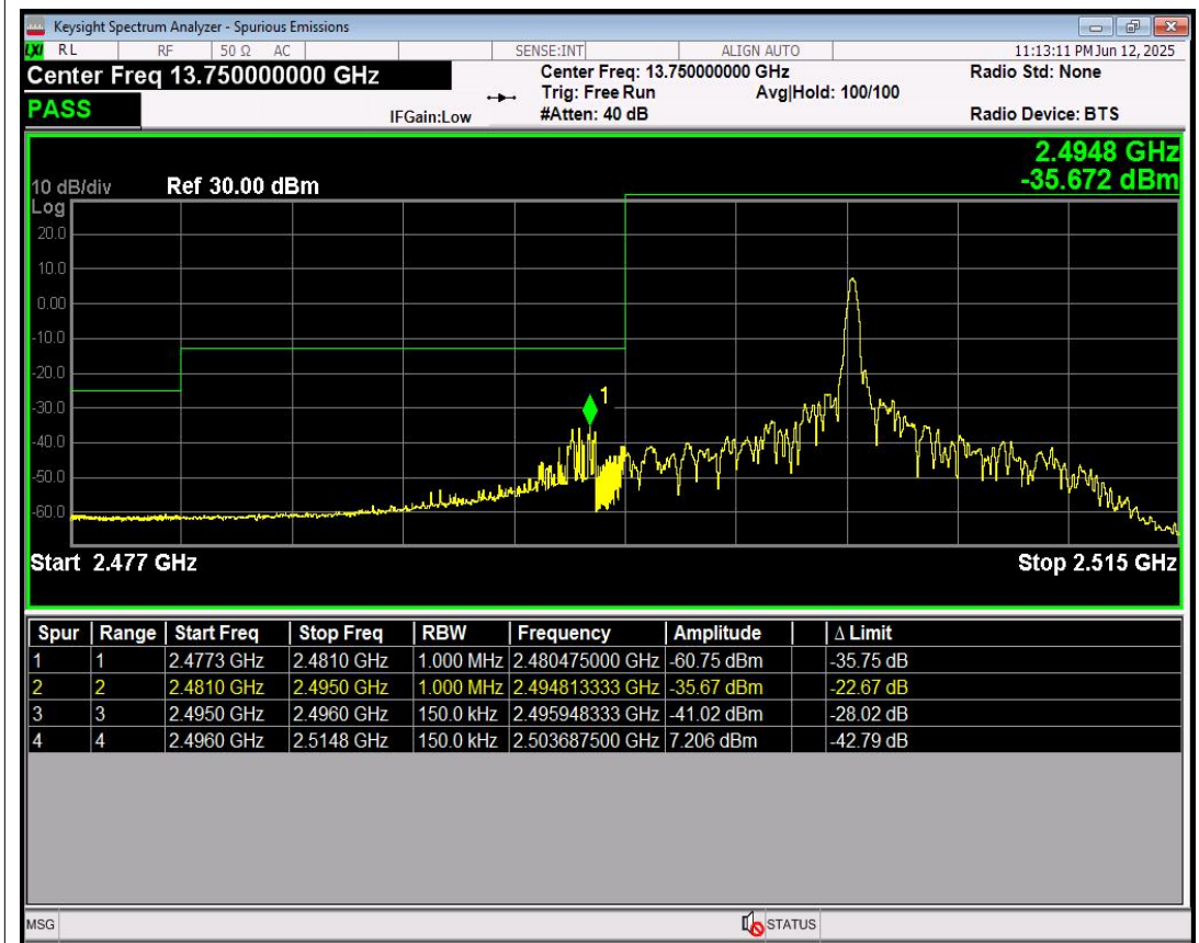
Band41 QPSK BW=15MHz Channel=39725 RB Size=1 Position=#Mid
