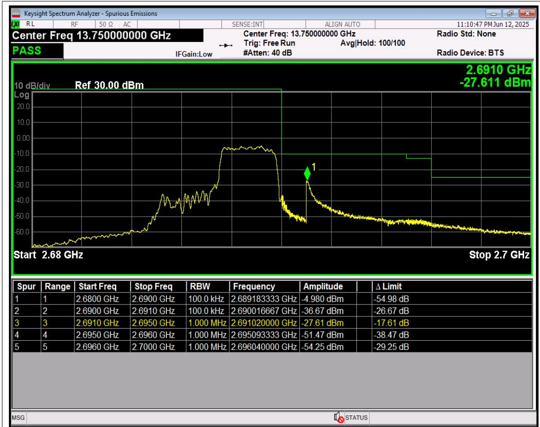
Band41 QPSK BW=5MHz Channel=41565 RB Size=12 Position=#Max
