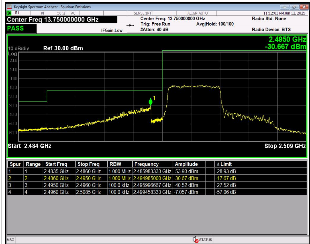
Band41 16QAM BW=10MHz Channel=39700 RB Size=25 Position=#0
