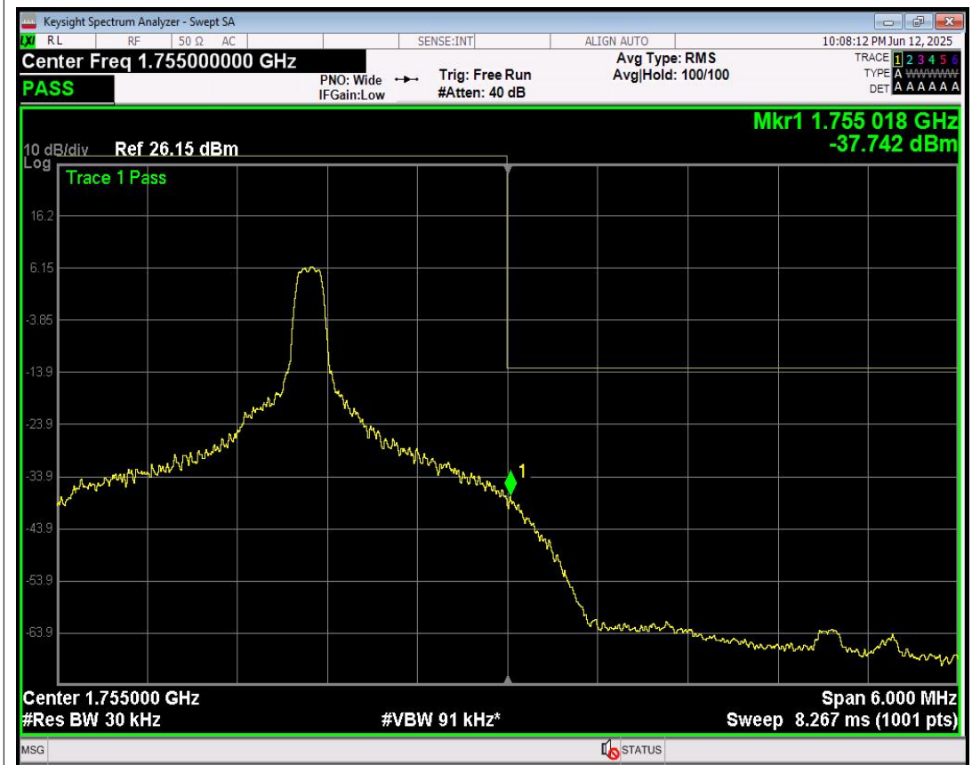
Band4 QPSK BW=3MHz Channel=20385 RB Size=1 Position=#Mid
