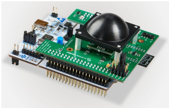
Figure 1 Evaluation kit SiRad Easy® with assembled lens
