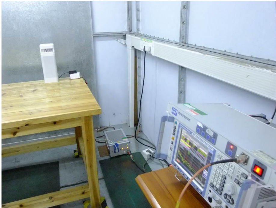
Test Setup For Conducted Emission
