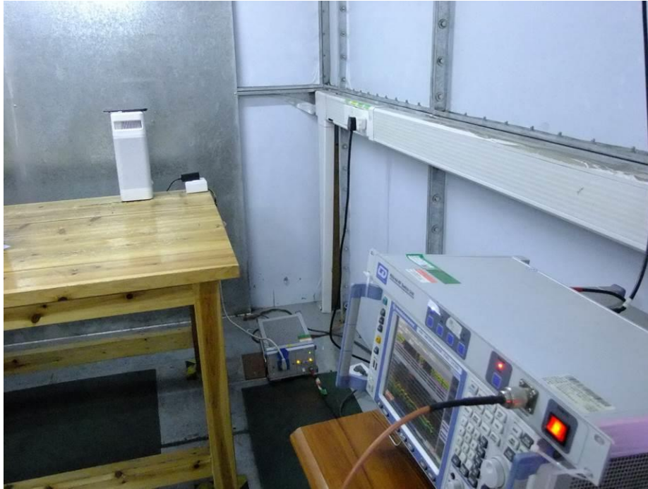
Test Setup For Conducted Emission
