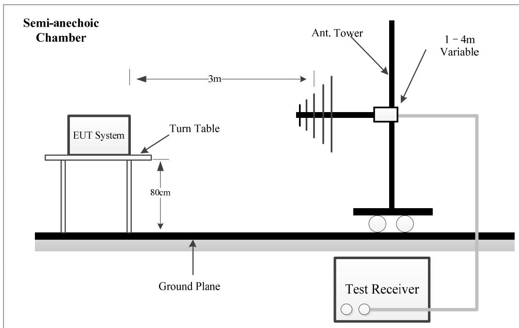
The radiated emission tests were performed in the 3-meter chamber test site, using the setup accordance with the ANSI C63.10-2020.
