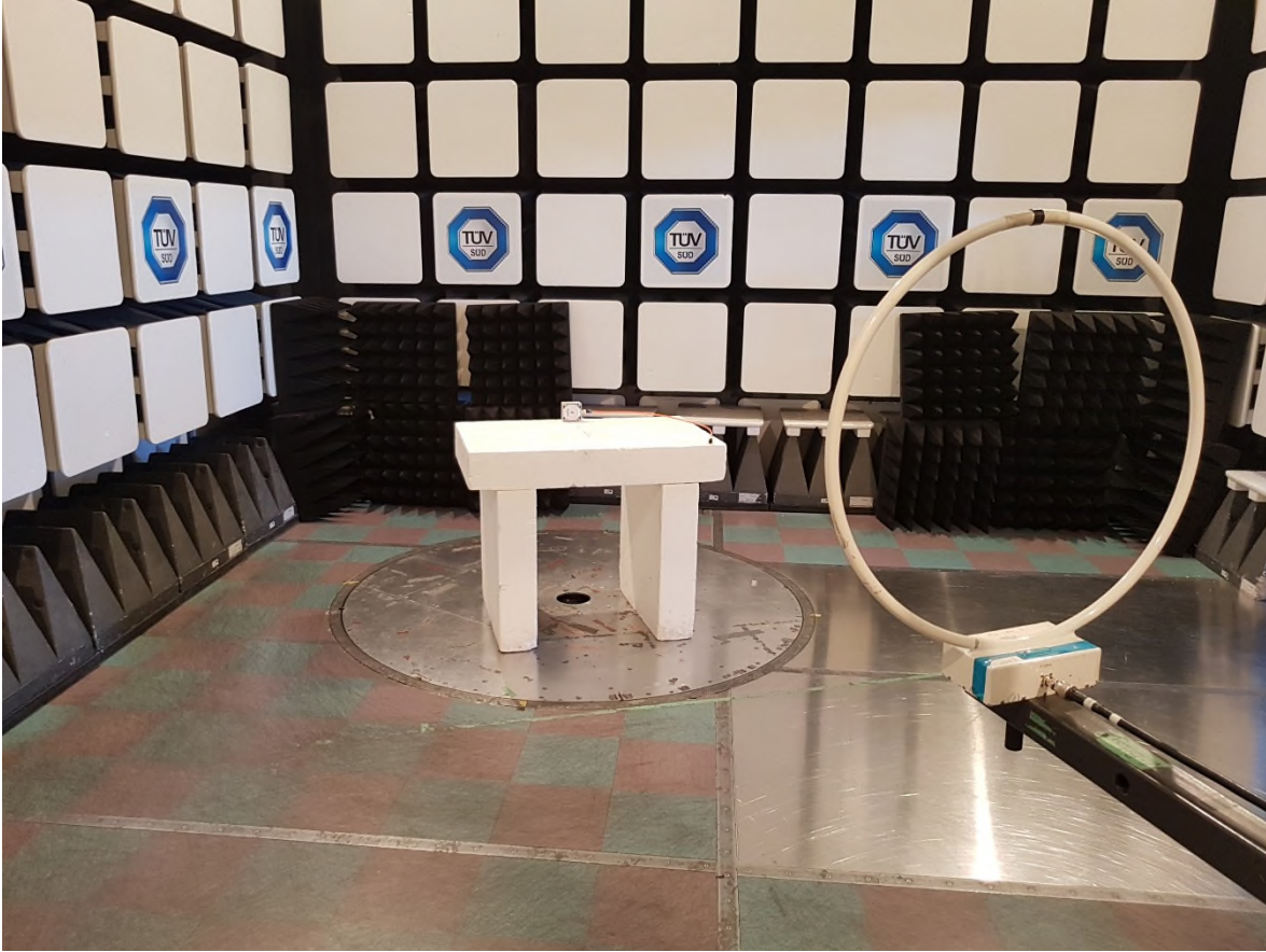
Figure 3 – Radiated Emissions Setup
