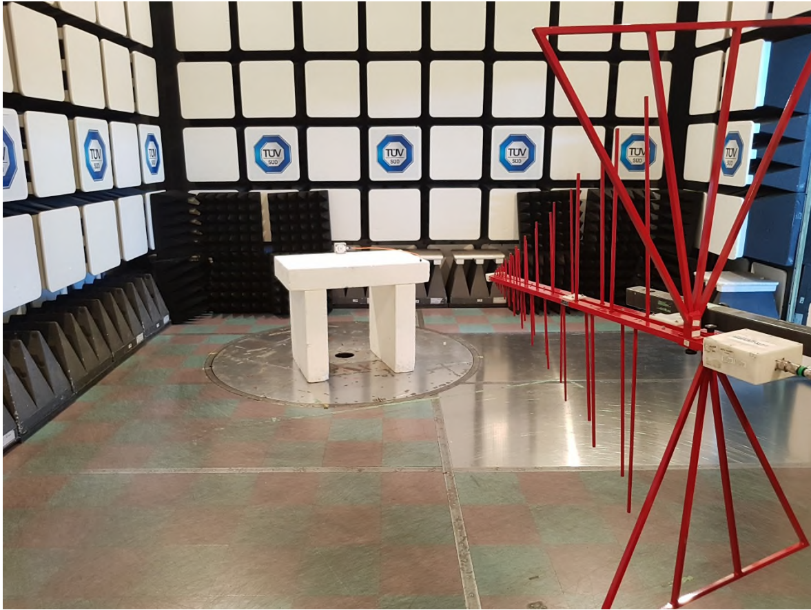
Figure 4 – Radiated Emissions Setup
