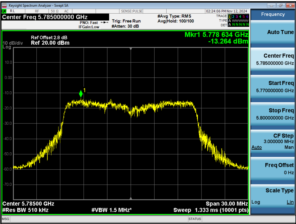
PSD NVNT a 5785MHz Ant1
