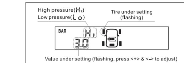
Setting items: Pressure unit – Temperature unit – Front tires pressure threshold – Rear tires pressure threshold ...
