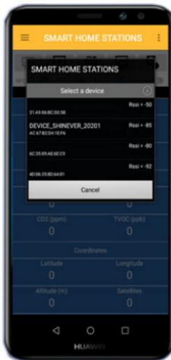
**The Smart Home Stations** device will be listed in the BLE device list as an item started with “DEVICE\_SHS” and followed by SHS version number and other small version numbers.
