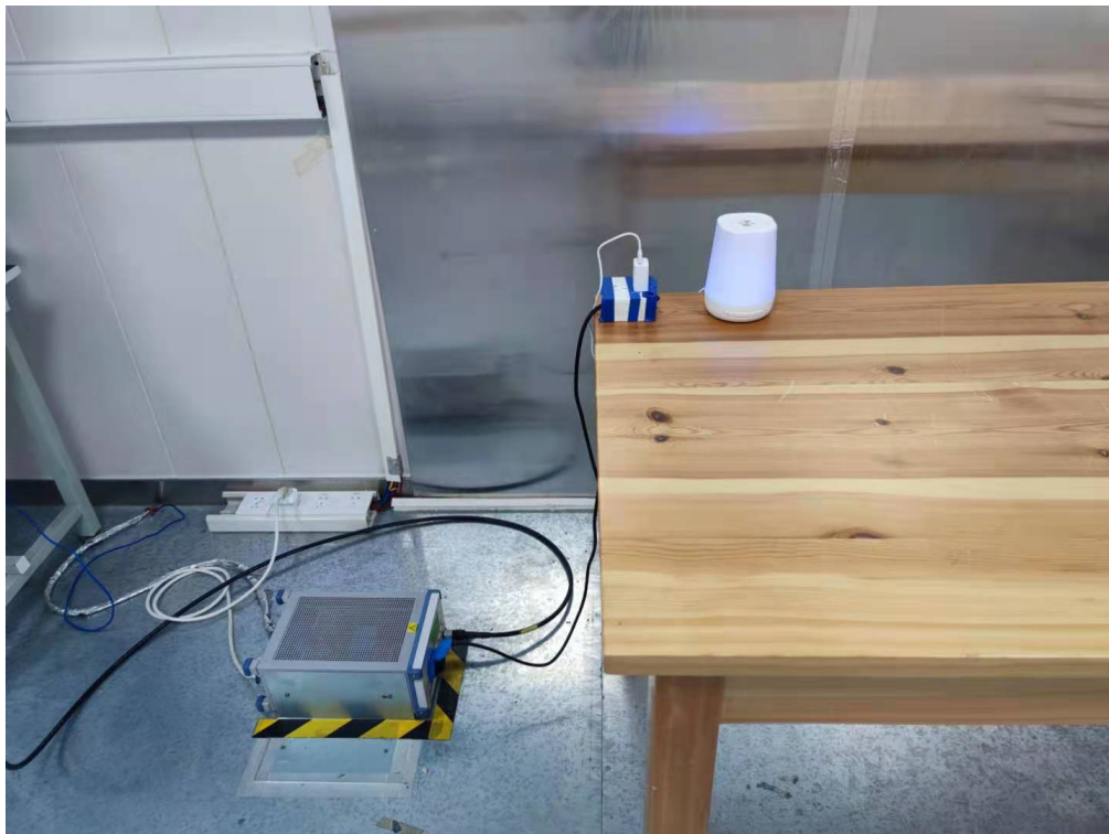
Above 1GHz for radiated emission test setup
