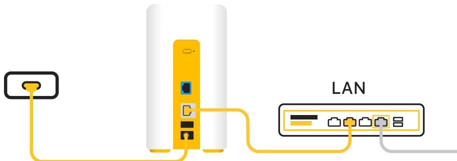
Use an ethernet cable to connect the Firewalla AP7 with a Firewalla Router, and plug the AP to a power source.
