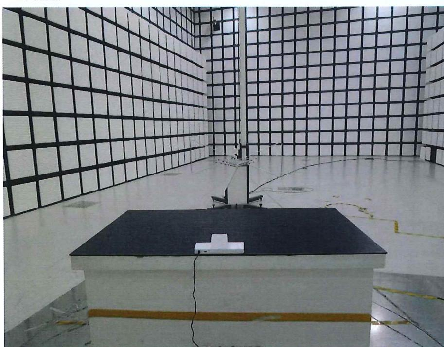
2. Radiated Emission setup photo (Above 1 GHz)
