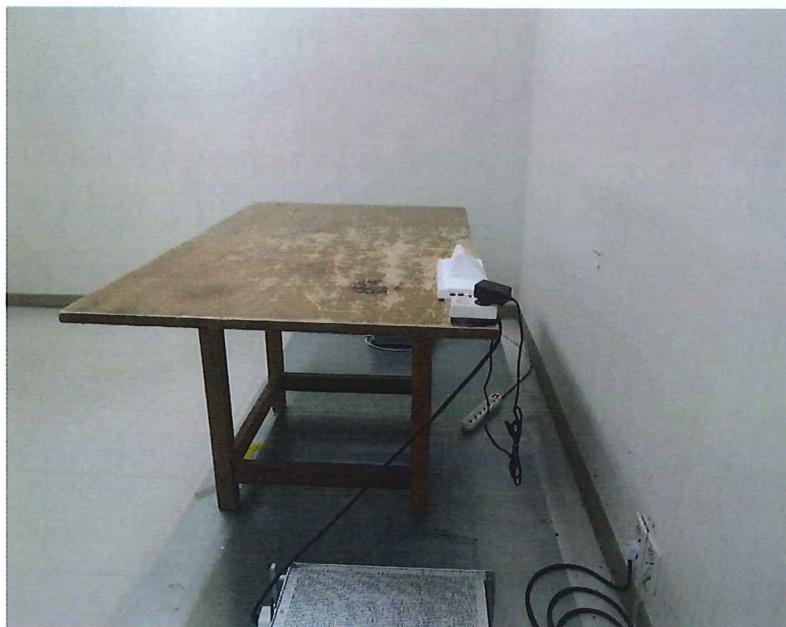
1. Radiated Emission setup photo (below 1 GHz)
