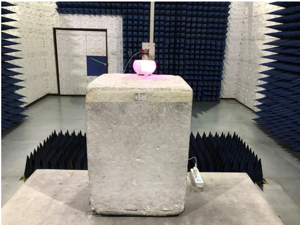
RADIATED EMISSION TEST SETUP ABOVE 1GHz
