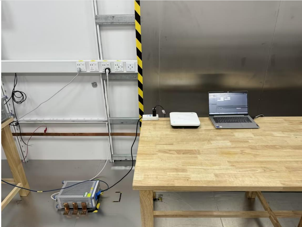
AC Power Line Conducted Emission
