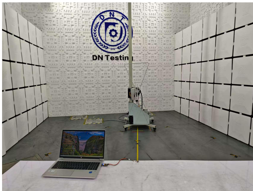
Radiated Emission Test View|(Below 1G)
