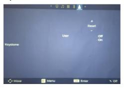
In ladder correction, you can set and select ladder correction+or-, and press the up and down keys on the remote control to correct the screen image.
