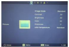
You can select the image mode using the upper / bottom button In the display settings, you can set the brightness (+ / -), contrast (+ / -), saturation (+ / -), and sharpness (+ / -). After selection, press OK to confirm.
