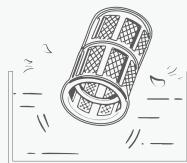
3 Wipe the filter screen and place it back into the fuel.
