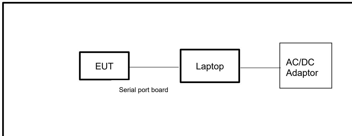
Note: AC/DC Adaptor is used for AC conducted power line test only.
