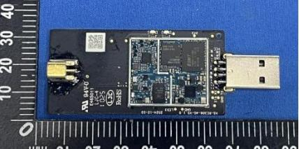
A photograph of the modified PCB. The antenna has been removed, and a new antenna interface is visible. A metric ruler is placed next to it for scale, showing 10, 20, 30, and 40 mm. Below the PCB, a separate image shows the removed antenna and a new antenna cable. |
