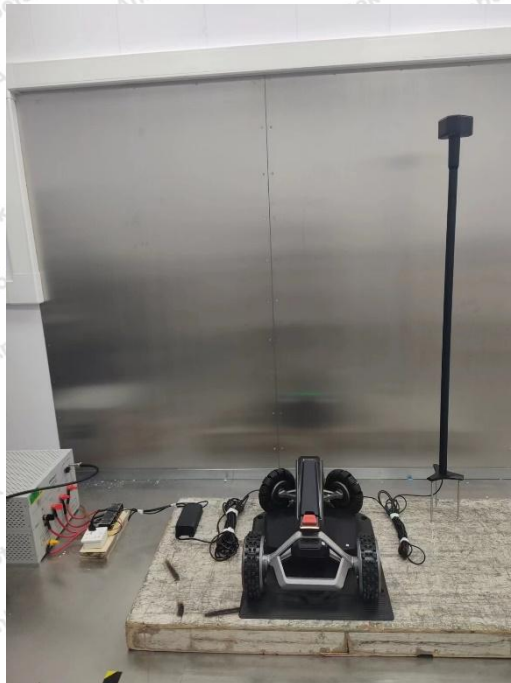
Photo of Conducted Emission Measurement
