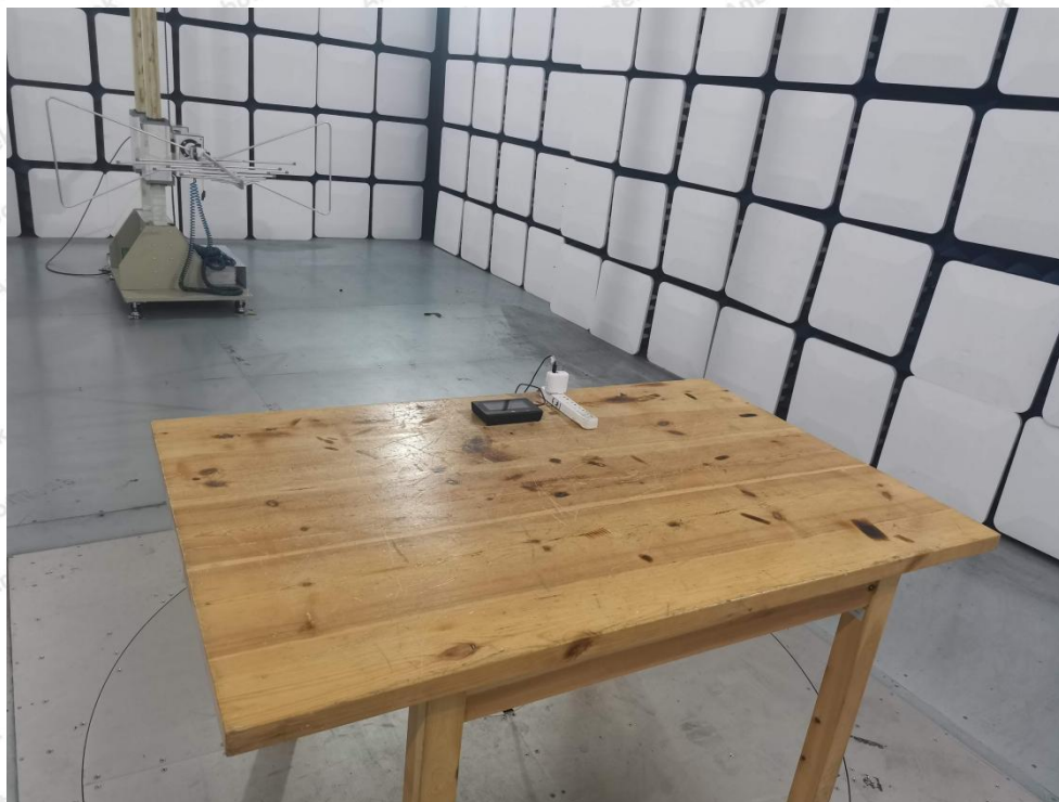
Photo of Radiation Emission Test
