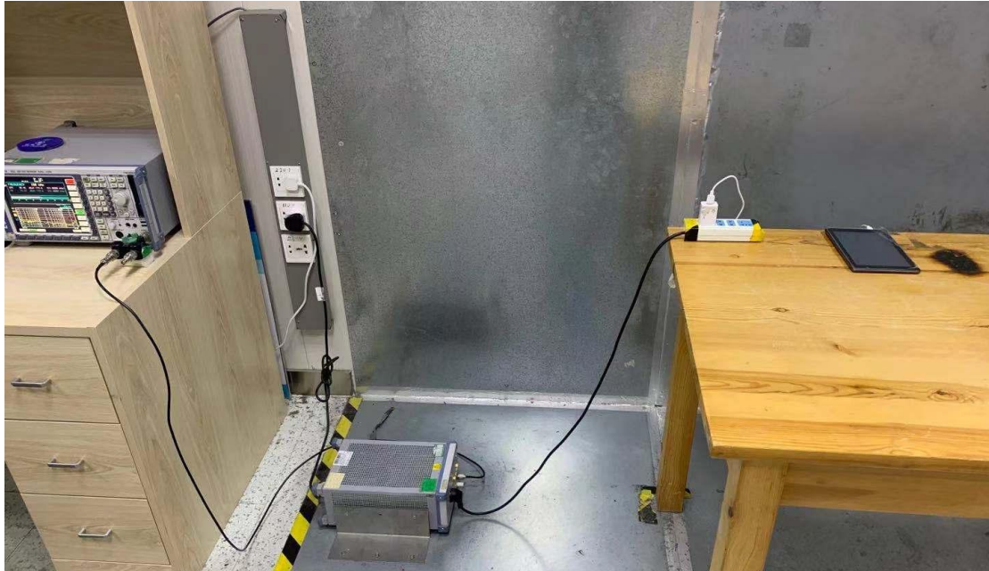
Radiated Spurious Emissions From 30MHz-1000MHz
