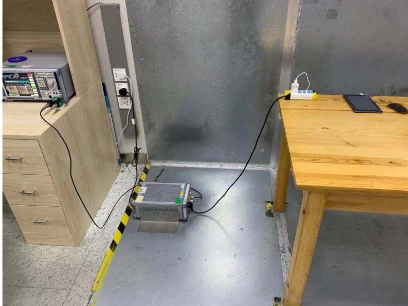
Radiated Spurious Emissions Test Frequency From 30MHz-1000MHz
