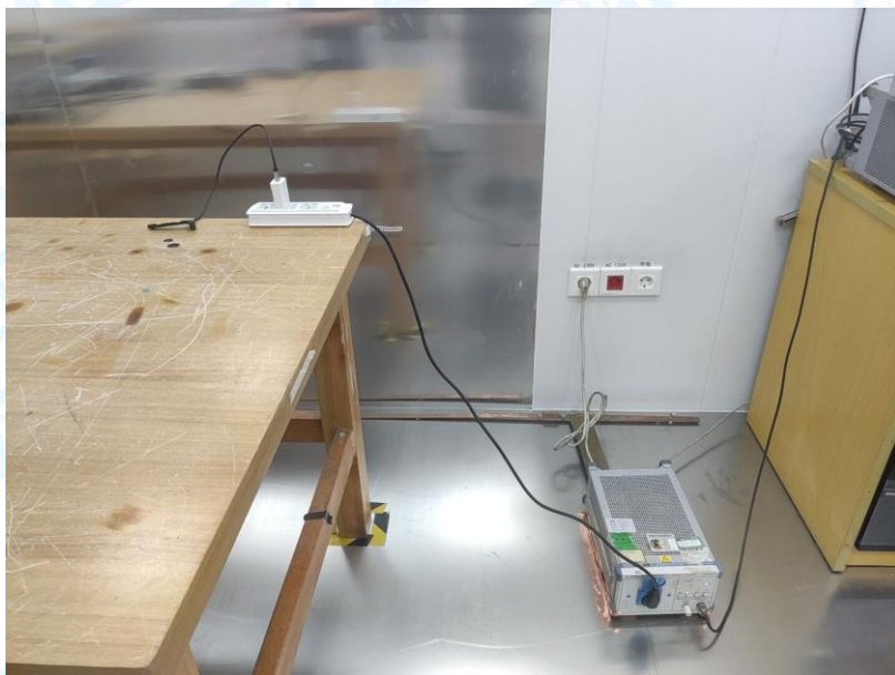
Photo of Setup for Conducted Emission
