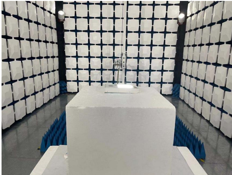
Below 1GHz for radiated emission test setup
