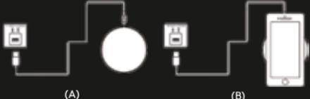
Use the charging cable provided to charge the wireless base. Connect the type C input to the base and the USB-A output to a wall charger or to a computer. (A)
