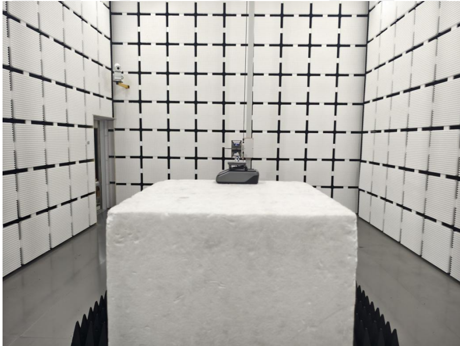
Spurious Radiation Emissions Test (>1G)
