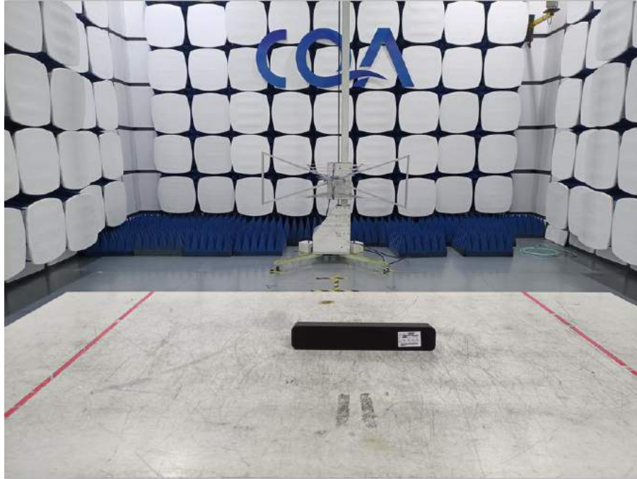
Radiated Emission Test Setup
