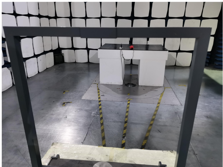
Radiation Emission Test Setup (Below 30MHz)
