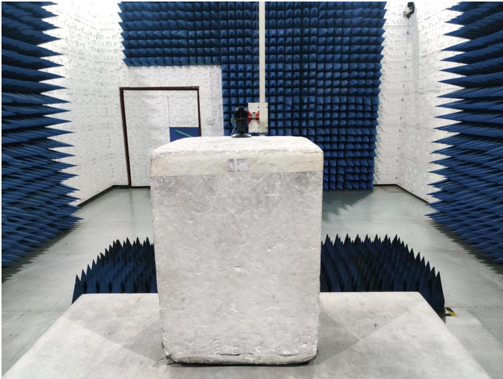
FCC RADIATED EMISSION TEST SETUP ABOVE 1GHZ
