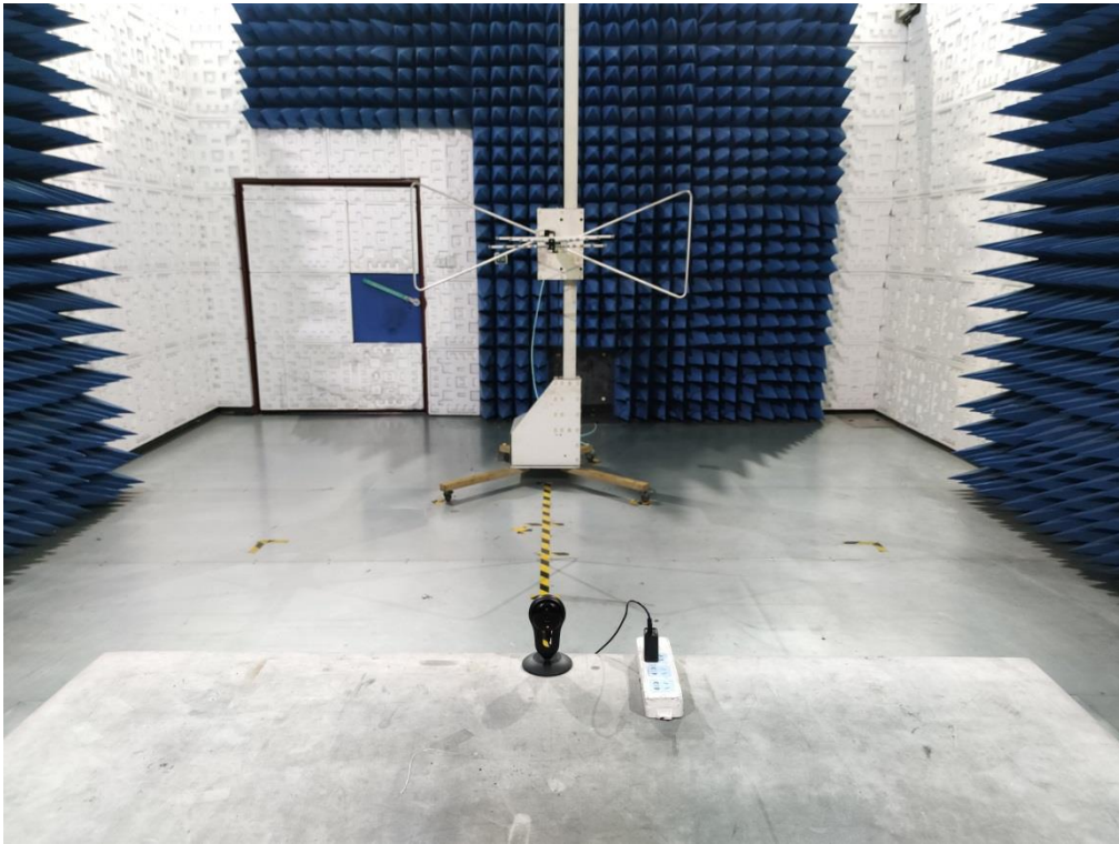
FCC RADIATED EMISSION TEST SETUP ABOVE 1GHZ
