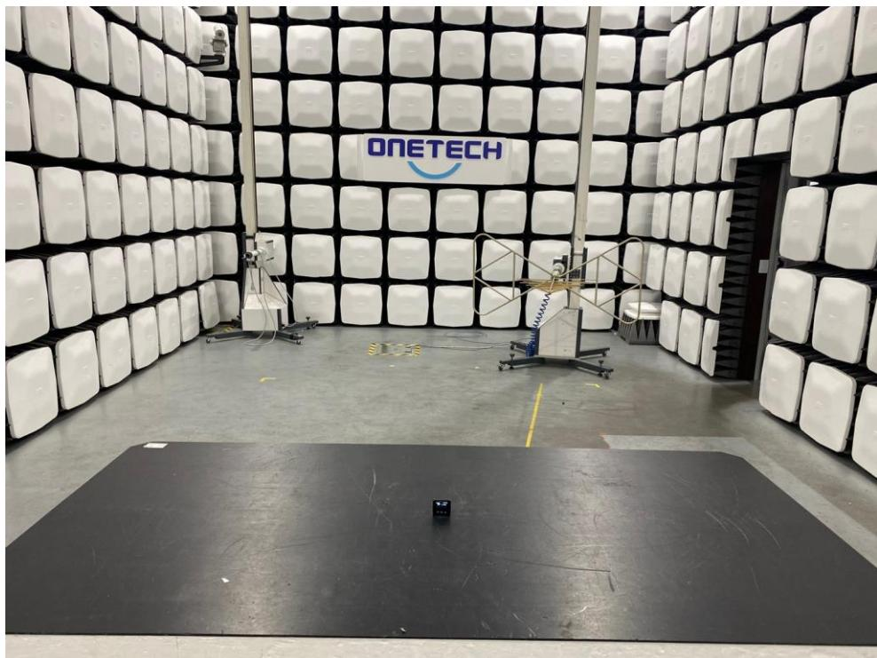
**- Radiated Emission Test (Above 1 GHz)**
