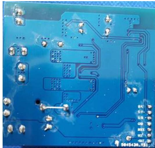
The electronic board is used for kid car, and controls kid car to move forward, move back, swing. Also, can adjust speed accordingly. Power by battery to drive motor, turn via motor too.
