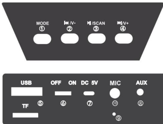
1. MODE Short press for switching BLUETOOTH,TF CARD,USB,AUX,FM Radio mode.
