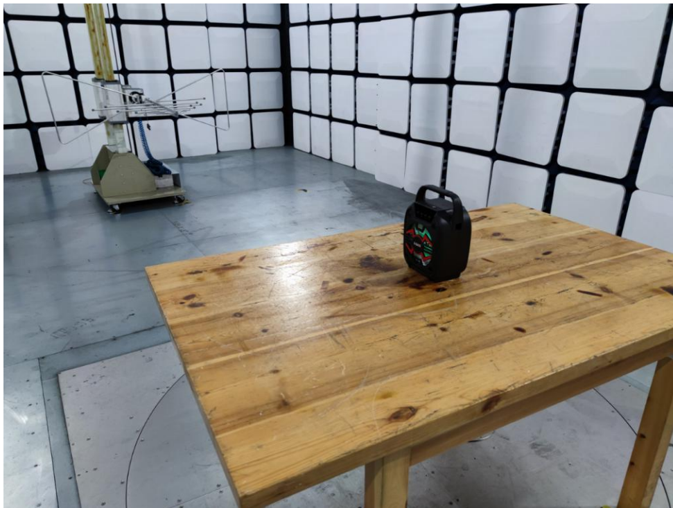
Photo of Radiation Emission Test
