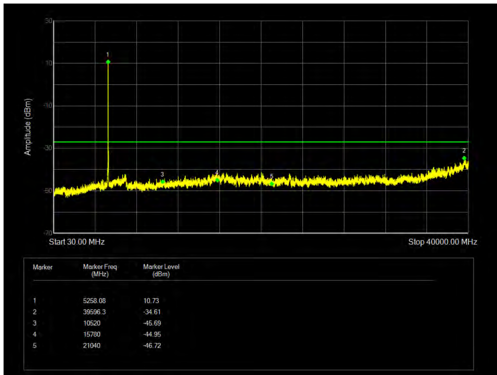
Tx. Spurious NVNT 802.11ac20 5280MHz Ant1 Emission
