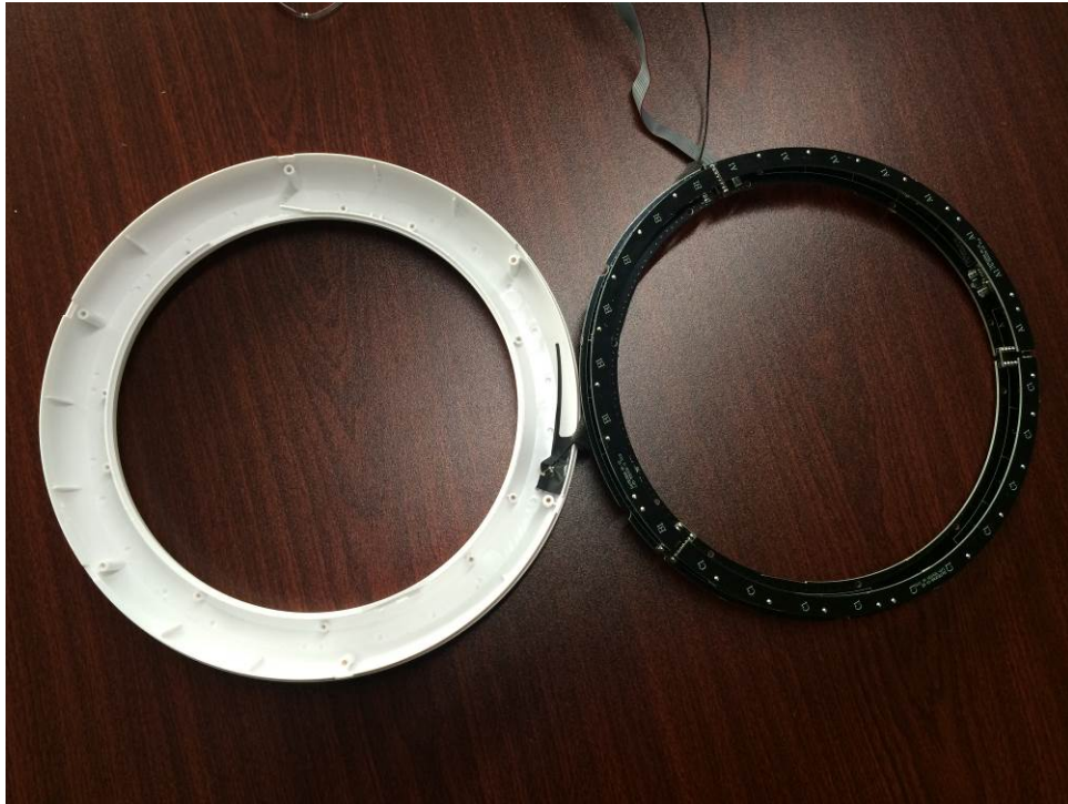
Figure 21. Control PCB view
