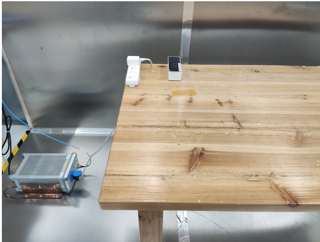
Photograph 3: Set-up for Conducted Emission on AC Mains
