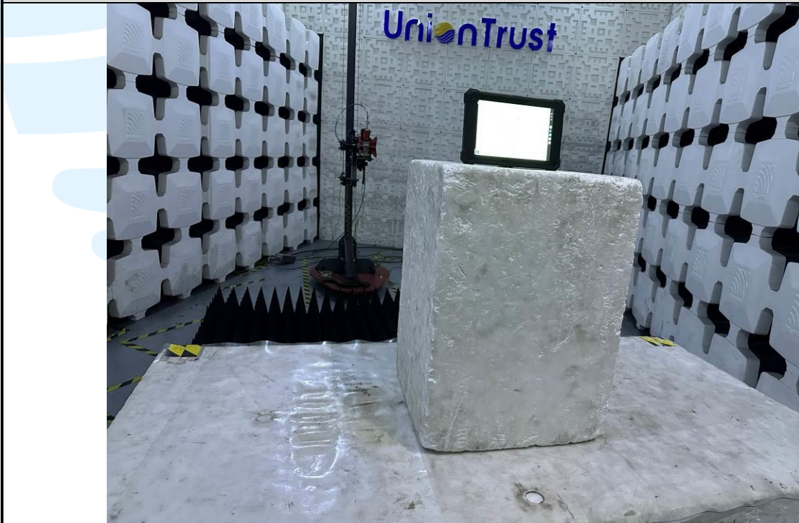
Radiated emission Test Setup (Above 1 GHz)
