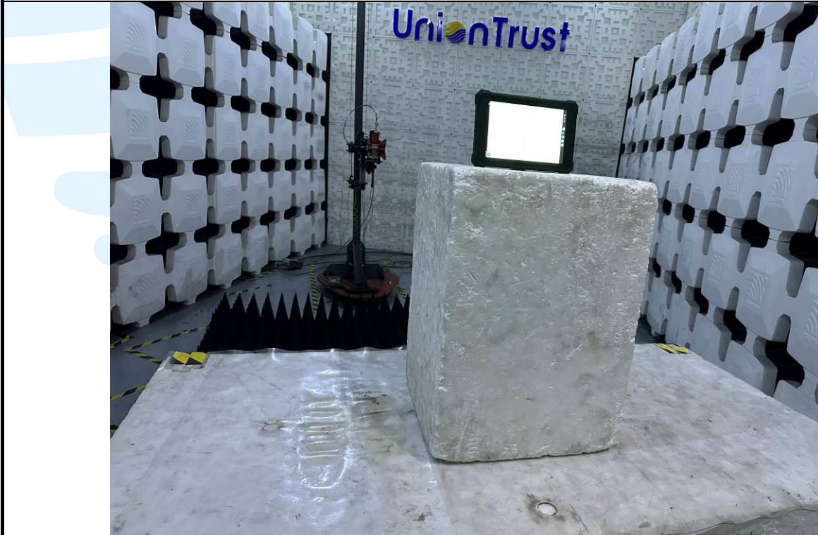
Radiated emission Test Setup (Above 1 GHz)
