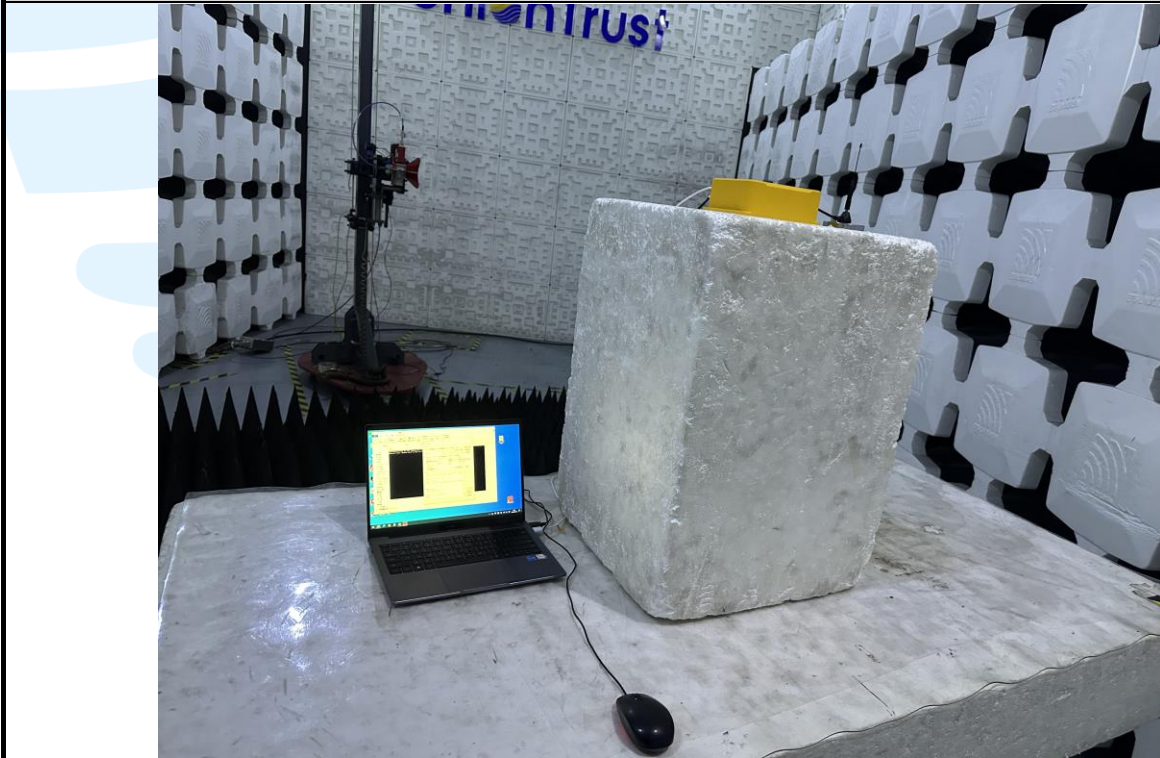
Radiated emission Test Setup (Above 1 GHz)
