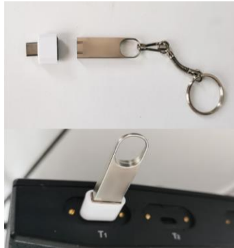
Figure 3.7.9 Connection diagram of mobile storage device
