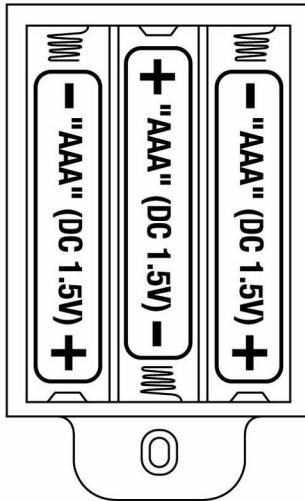
Install 3 AAA batteries into Spybot as shown
