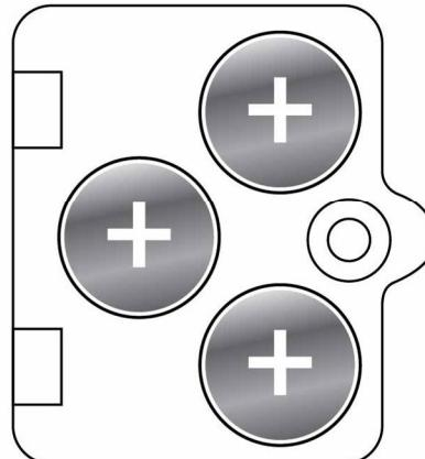
Install 3 button cell batteries into backpack as shown.
